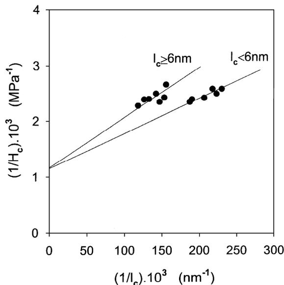
Fig. 2. Plot of  $H_c^{-1}$  as a function of  $l_c^{-1}$  for atmospheric pressure crystallized PEN.
