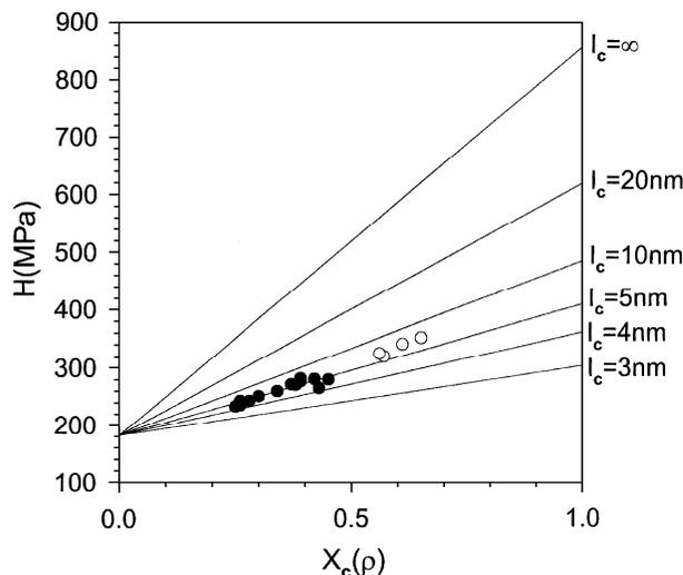
Fig. 3.  $H$  variation with  $X_c$  for atmospheric (solid symbols) and high-pressure (open symbols) crystallized PEN. The straight lines follow Eq. (7) (see text).
